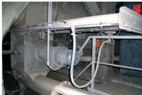
FLUIDCON transport system at Holcom Plant Lägerdorf for 230 t/h cement.
