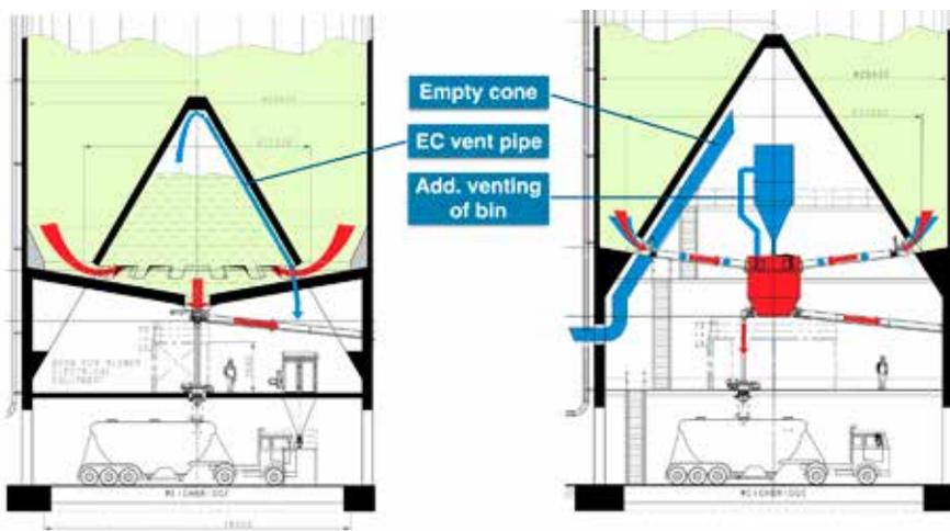
Figure 3. Technical comparison: operational behaviours of air and cement flow of an EC silo (left) and ME silo (right).
