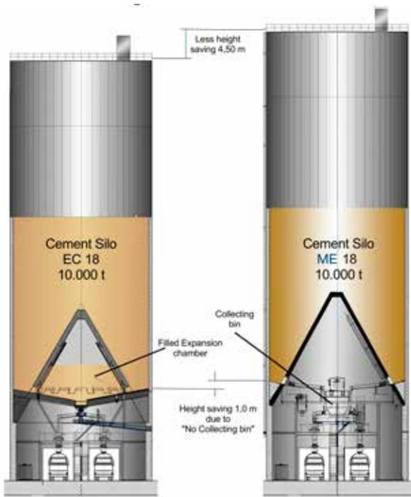
Figure 4. Technical comparison: construction and design of an EC silo (left) and ME silo (right).
