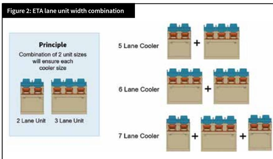
In terms of cooler length, by combining 3.3m- and 4.4m-long units, the cooler can be replaced with an accuracy of 1.1m in length.
