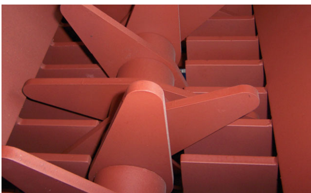
Detail of breaker and grid
