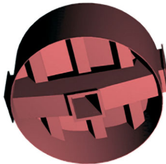
Discharge tunnel under silo cone leads to continuous discharge conditions at outlet
