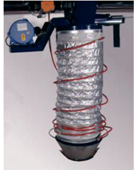
Stationary loading device
