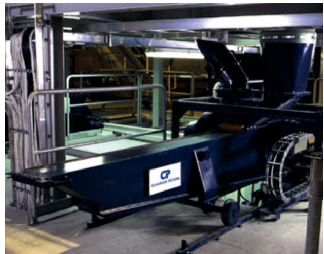
Mobile Loader with travelling ranges between 1 and 15 m
