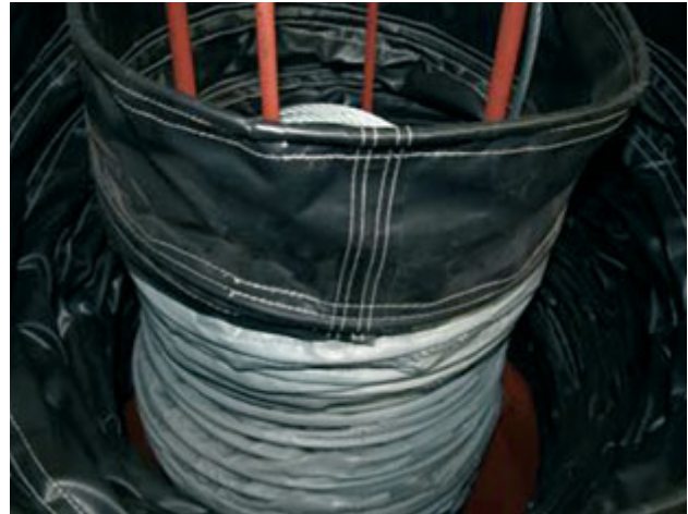
Loading device with outer and inner bellow for standard materials (e.g. cement)
