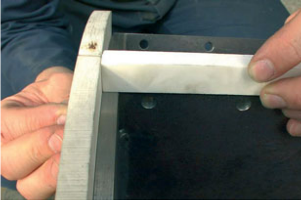
Installation of ceramic elements at rotor perimeter
