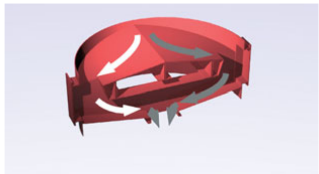
Discharge tunnel to center outlet
