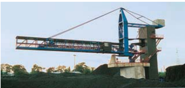
Coal stacker at a power station
