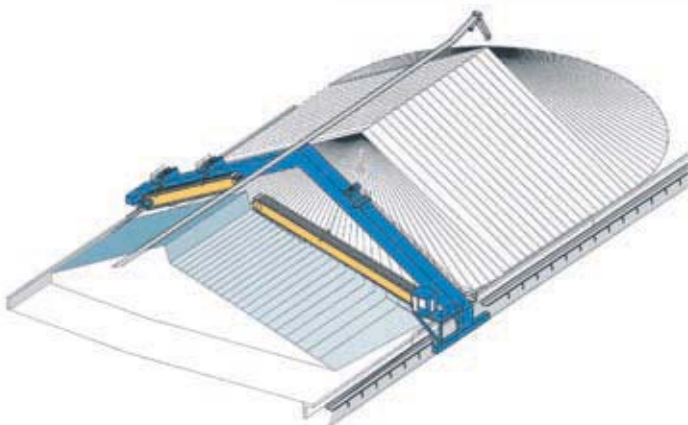
Longitudinal stockyard with twin-boom portal reclaimer
