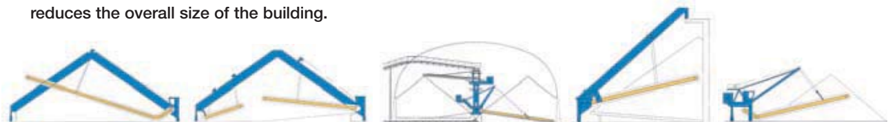
Single-boom portal reclaimer
