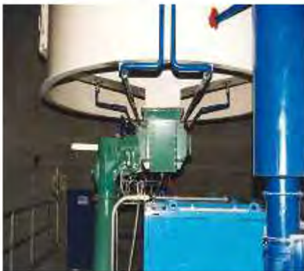
Discharge tunnel under silo cone leads to continuous discharge conditions at outlet
