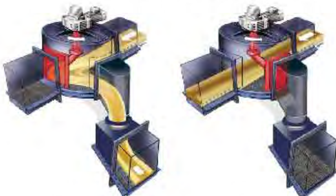
Operation principle of Claudius Peters Two-Way Gate, used as bottom discharger
