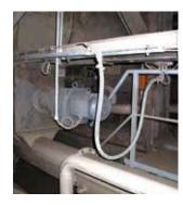
Rotary Feeder with FLUIDCON.
