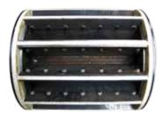
Installed rotor cell with ceramic wear elements.
