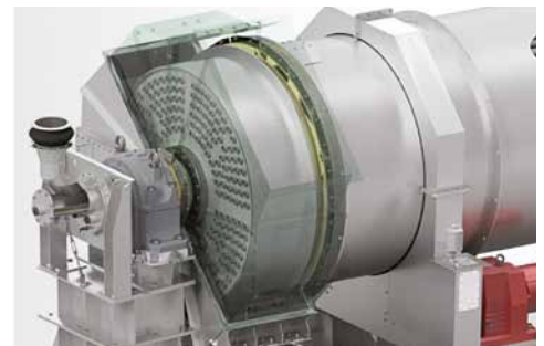
The VFD controlled fan drive motor grants a constant stucco temperature for all seasons and temperature fluctuations.
