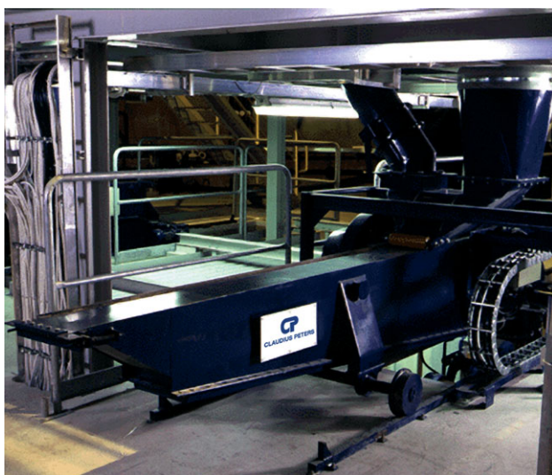
Mobile loader with traveling ranges between 1 and 15 m
