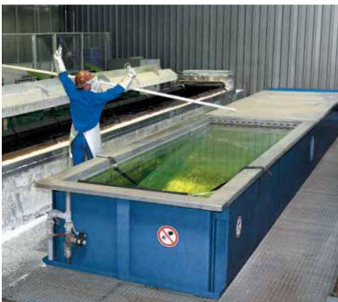
Lifting from the salt bath and quenching in the tempering bath.
