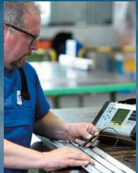
HFEC Surface Crack Testing.
