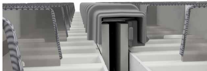
Schematic representation of the ETA cooler lanes (left: sectional view lane of previous ETA generation; right: sectional view of newest ETA generation).
